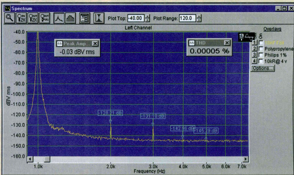
Figure 8: The makers replacement extended foil/Polypropylene shows the same 0.00005% distortion but second harmonic is 1dB worse. With test signals increased to 6 volts and DC bias to 30 volts second harmonic increased just over 5dB, distortion to 0.00008%. Again, no visible intermodulation.
