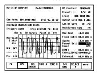
The System Analyzer includes the capability of encoding and decoding PRIVATE LINE (DPL), DIGITAL PRIVATE LINE (DPL) and single tone sequences as well as multi-tone sequences including DTMF signals, 5/6 tone paging, Select V and up to 20 sequential tones. Decoding displays include tone frequencies and time durations of the individual tones. The unit can also encode tone remote signaling.
