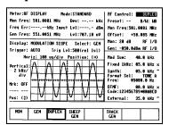
Full output level control from -130 dBm to 0 dBm over the entire range of the instrument is available from the RF I/O port (-130 dBm up to -50 dBm) and the generator port (-80 dBm to 0 dBm). Variable offsets from 0 to +/-55 MHz in 5 kHz steps are keypad selectable.
