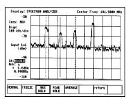
The built-in Spectrum Analyzer of the R-2600 will display a window of RF spectrum anywhere within the 400 kHz to 1GHz operating range of the unit. The EXPAND soft key enlarges the display to fill the CRT and retains complete audio, dispersion and center frequency control.
