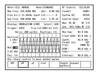
Convenient channel number entry sets up the unit for manual testing. Subscriber radio must be put into its internally controlled manual test mode.
