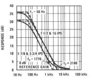
FIGURE 8. NAB Equilization Characteristic
