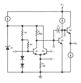
FIGURE 3. AC Equivalent Circuit
