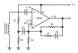
FIGURE 11. Fast Turn-On NAB Tape Preamp.
