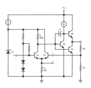
FIGURE 4. Differential Input Biasing
