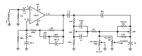
FIGURE 23. Single Channel of Complete Phono Preamp.
