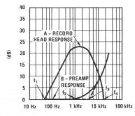
FIGURE 15. Recording Head & Preamp. Response for NAB Equilization
