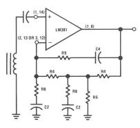
FIGURE 12. Two-Pole Fast Turn-On NAB Tape Preamp.
