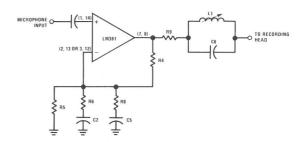
FIGURE 16. Tape Recording Preamp.
