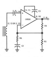
FIGURE 7. Flat Response Tape Amplifier
