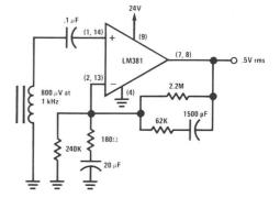
FIGURE 10. Typical Tape Playback Amplifier
