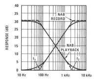
FIGURE 14. NAB Record & Playback Equilization
