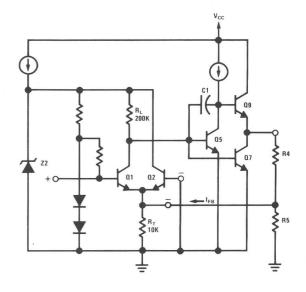
FIGURE 5. Single Ended Input Biasing
